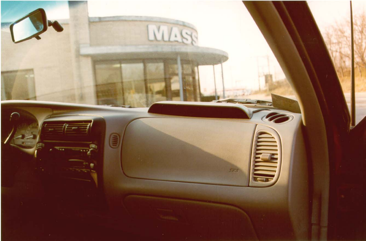
Photograph Showing the M-3009 Mounted on the Instrument Panel of a Test Car
