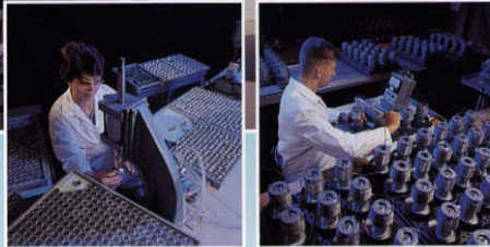
Assembly of TR-89 Air Ultrasonic Transducers and TR-208A/SQS-23 Sonar Transducers.
