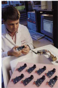
Electroacoustic Specialist checking preproduction assemblies of a Massa custom designed OEM Ultrasonic Control System.
