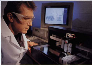
Electronic Engineer operating the Massa PC Board Rapid Prototyping Machine.
