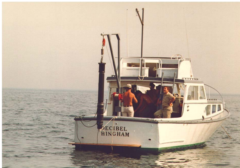
Fish Assembly Less Streamlined Housing of the Engineering Model of the M-1002 Portable Sonar System During Sea Test On-board the 38 ft. Research Vessel R/V Decibel
