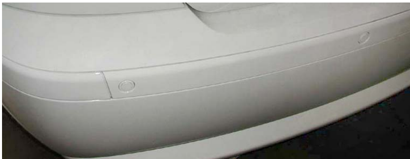
An Automobile Bumper Showing How It Appears with the Existing Transducers that Protrude Through the Bumper and Are Exposed
