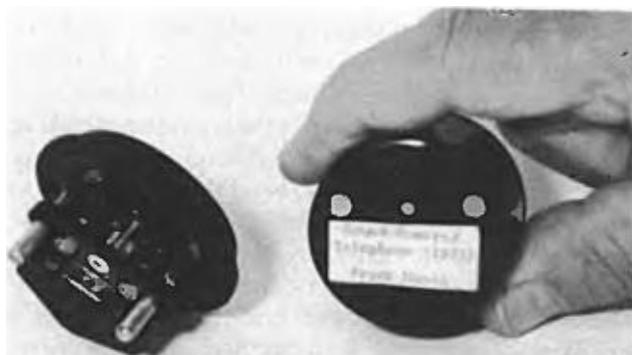
FIG. 13. High efficiency blast-proof sound powered telephone element (1933).
