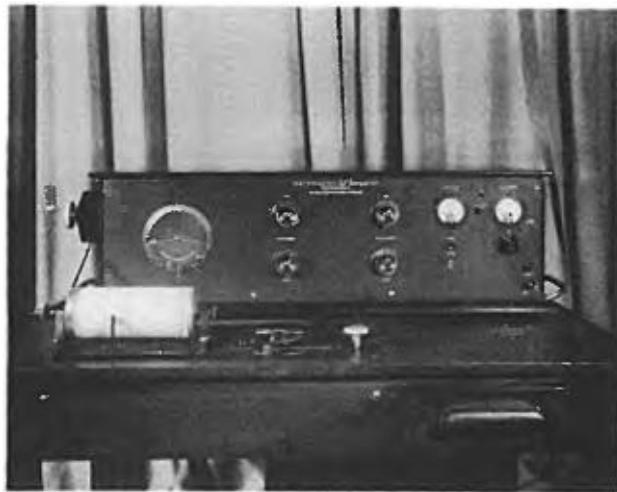
FIG. 1. Early beat frequency oscillator with logarithmic frequency scale and recording drum attachment for plotting frequency response characteristics of loudspeakers (1929).
