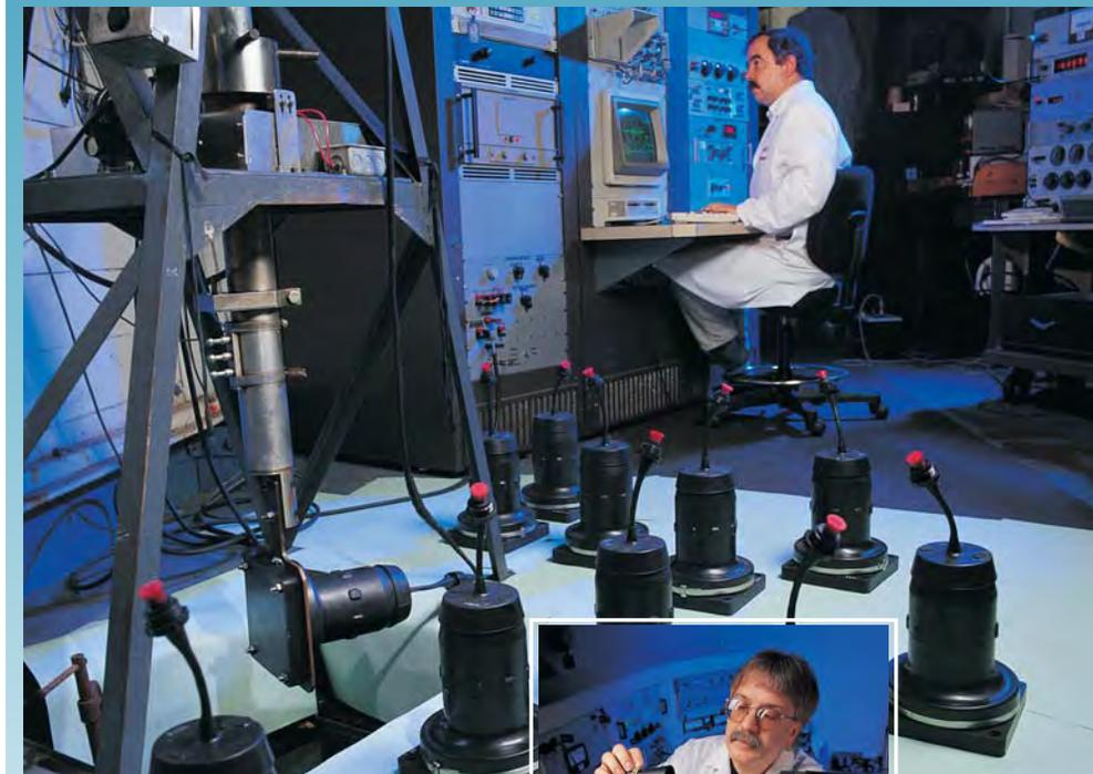
Sonar Transducer testing in the Underwater Test Pond at the Massa Facility.
