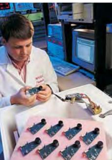
Electroacoustic Specialist checking preproduction assemblies of a Massa custom designed OEM Ultrasonic Control System.
