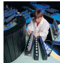
Various stages of assembly for a specialized Sonar Transducer Array.
