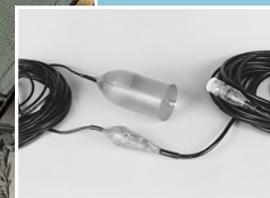
Towed array containing transducers and electronics redesigned and manufactured by Massa for the U.S. Navy (c. 1990).
