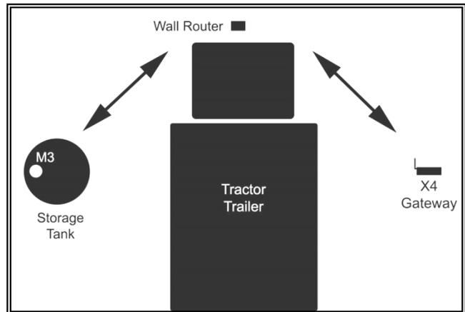
This example shows a much taller tank with a gateway placed high overhead. Here the tractor trailer does not impede the radio signals.
