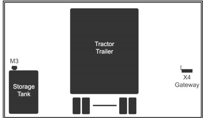
Placing a Digi Wall Router as shown will allow another path around metal structures that could block the radio signal. Simply plug in the wall router and they should associate and be listed on the Xbee Network as a *router* Node Type. You may also use wall routers to extend the range between gateway and sensors.
