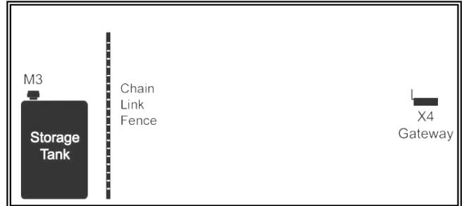
This scenario will also reduce the effective radio range. Place wall routers between the 2 points or place the gateway closer to the storage tanks. The radio signals here can bounce away from the sensor if the roof is metal.
