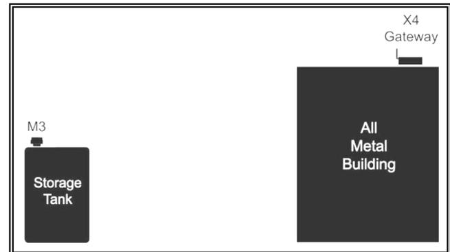
This scenario has the gateway antenna at the same level as the SonAire M3 Sensor mounted on metal storage tanks. The RF signal may skip off the closer tanks and poor signal levels may occur at the further tanks. Raising the gateway's antenna will improve the signal to the further tanks.
